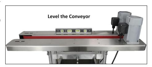
If adjustments are required, loosen the height adjustment nuts on the feet of the conveyor with a  $15/16^{th}$  wrench.
