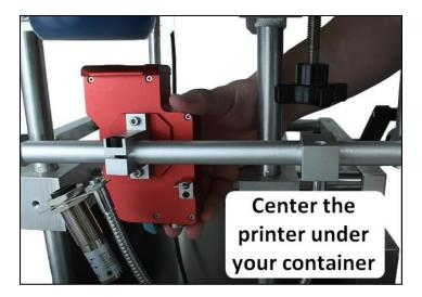
12. Position the sensor so it is slightly upstream of the printer and pointing directly at the container in the conveyor.
