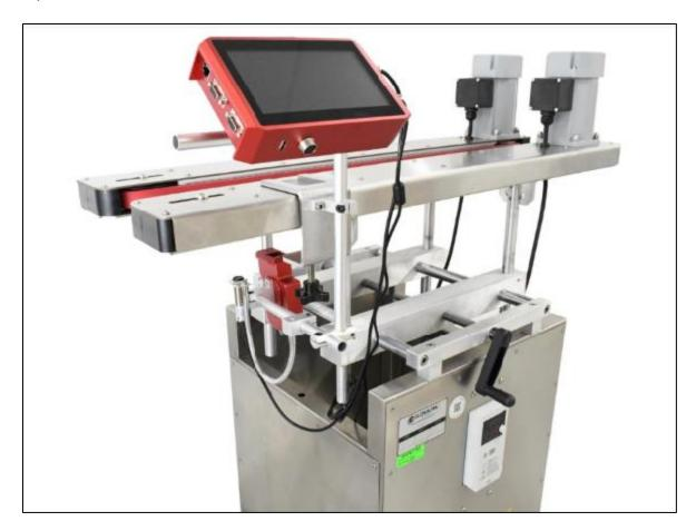
This is just one possible setup for the inkjet printer, where it is set up to label the bottom of standard bottles. However, the rod mounting system is highly adjustable and can accommodate many different containers and printing locations. Do not hesitate to modify your setup based on your needs.
