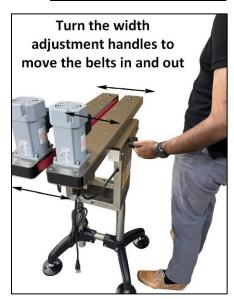
3. Use one of your containers to make the necessary adjustments to your belt width. Widen the belts so that the container fits between them, then shrink the gap once more so that the belts lightly squeeze but do not deform, your container. When you let go of the container, the belts should hold it in place.
