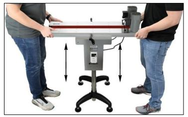
4. Position the bottomless conveyor cassettes so that they rest at the approximate center of a container sitting on your inline conveyor. When satisfied with the height of your bottomless, retighten the screws in the bottomless conveyor leg assemblies to lock the height in place.
