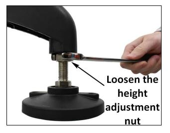
With the height adjustment nut loose, rotate the foot jam nut with a 7/8<sup>th</sup> wrench. To raise the conveyor, rotate the foot jam nut clockwise. To lower the conveyor, rotate the foot jam nut counterclockwise.
