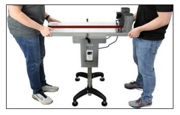
conveyor is lifted. Both carriers should stand on opposite ends of the conveyor, placing their hands under the corners of the deck, as shown in the image to the right.
