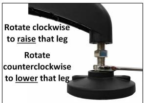
When the conveyor is at the desired height, tighten the height adjustment nut against the leg of the conveyor with a 15/16<sup>th</sup> wrench.
