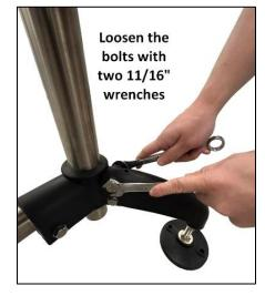
When the both leg assemblies have been loosened, two operators can lift and adjust the height of the conveyor.
