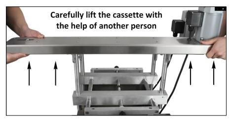
Adjust the cassette so that it is pointing at the approximate middle of a container sitting on your belt, as shown in the picture to the right. When you feel it is in the right place, retighten the set screws to lock the cassette height in place.
