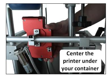
Position the sensor so it is slightly upstream of the printer and pointing directly at the container in the conveyor.
