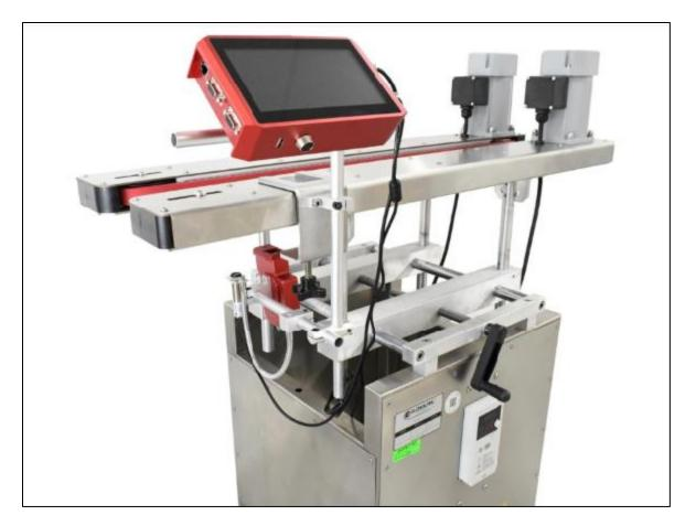
This is just one possible setup for the inkjet printer, where it is set up to label the bottom of standard bottles. However, the rod mounting system is highly adjustable and can accommodate many different containers and printing locations. Do not hesitate to modify your setup based on your needs.
