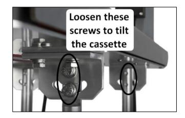
2. Once the bolts have been loosened, the belt cassette will be able to tilt about 45 degrees in either direction, as shown in the image to the right. Tilt the cassette to your desired location.
