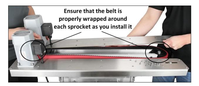
7. Push the top plate back onto the body of the cassette, ensuring that the belt is packed away nicely inside. Have one operator line up the holes in the top plate and hold the plate in place while the other begins reinserting the hardware, starting with the sprocket bolt.
