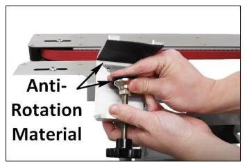
Fasten the printer clamp at the spot you would like for your printing to take place. We recommend mounting the clamp at the opposite end of the conveyor from the motors.
