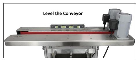
If adjustments are required, loosen the height adjustment nuts on the feet of the conveyor with a 15/16<sup>th</sup> wrench. Loosen the height adjustment nuts on the feet of the conveyor with a 15/16<sup>th</sup> wrench.
