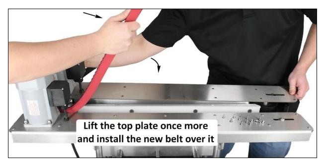
6. Once the belt is back underneath the metal of the top plate, ensure that it is properly wrapped around the sprockets in either end of the belt cassette.
